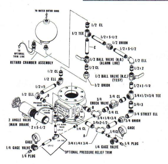
\*on 3" valves, substitute 1-1/2" fittings in place of 2" fittings shown.
